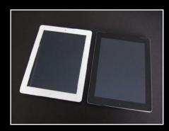
iPad 2: Apple's secondgeneration tablet computer, built thinner and lighter than the original while containing much faster processors and twin cameras for FaceTime. Comes in Wi-Fi-only or Wi-Fi + 3G versions, as well as white- or blackbezeled versions, each with silver aluminum backs.
