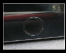
Touch ID Sensor: Apple's name for the fingerprint scanner debuted in the iPhone 5s, which rests below the Home Button and quickly scans fingers to determine whether to unlock the iPhone and allow iTunes Store purchases.
